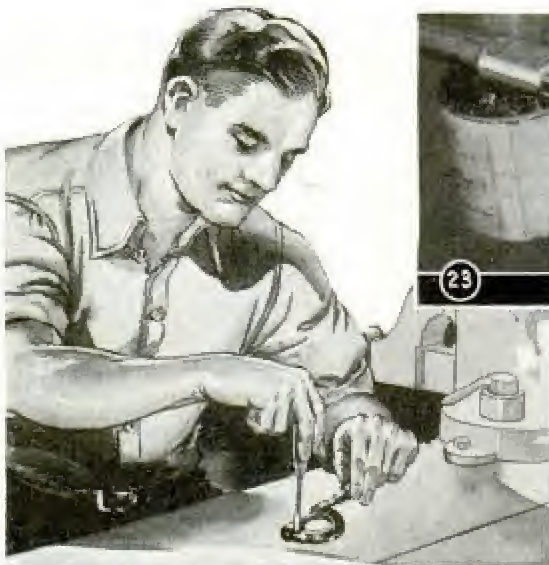
SQUARING WORN CONTACT OF MICROMETER SPINDLE
